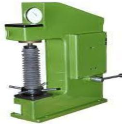
Fig.5. Shows the Rockwell hardness tester
