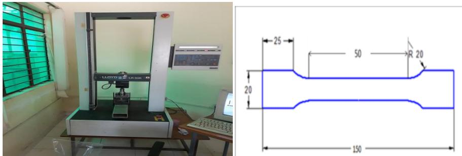
Fig. 3. Shows the UTM with tensile specimen
